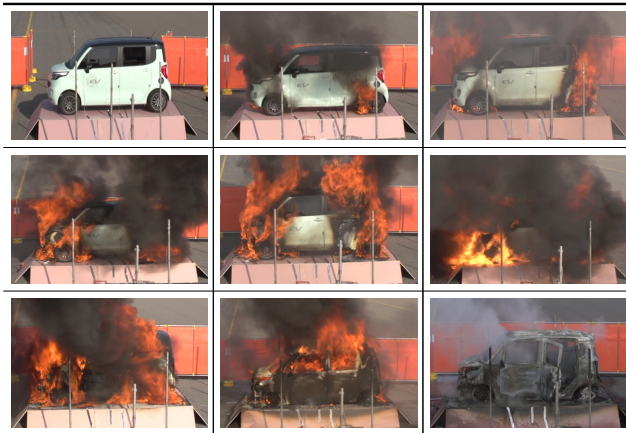
Fig. 6. Burning Process Picture of the Electric-Battery-Powered Vehicle
