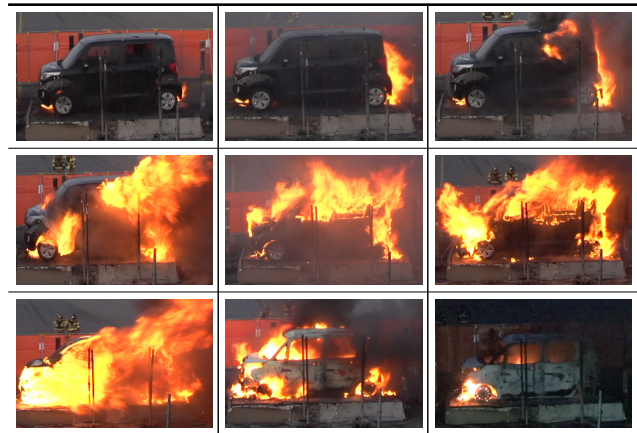
Fig. 4. Burning Process Picture of the Gasoline-Powered Vehicle
